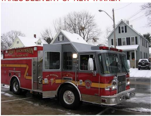
The Port Dickinson Fire Company recently took delivery of a KME 2005 pumper tanker, 2000 gpm, carrying 1800 gallons of water. The vehicle seats 6 and has a remote dump and closed circuit tv to monitor. The engine replaces a 1974Ward La France which will be sold. The vehicle was purchased with a Grant from FEMA.
